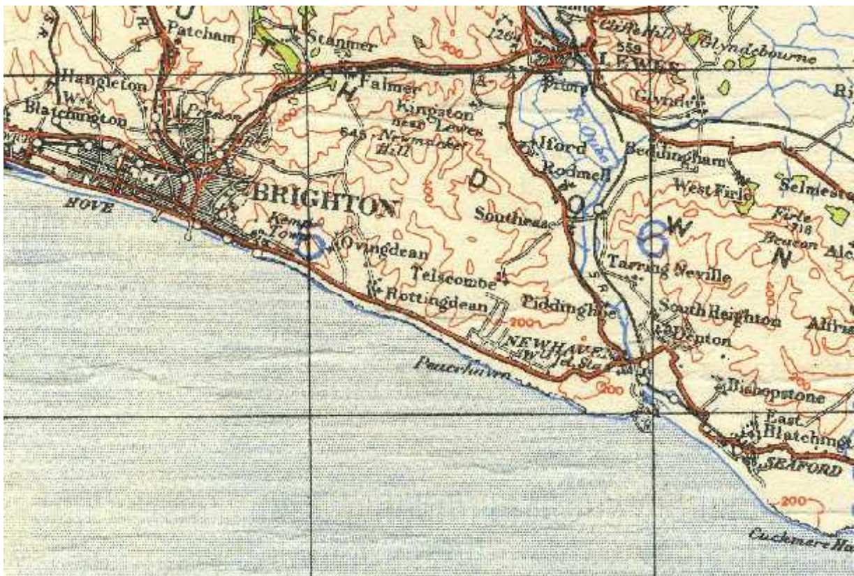
Extract from GSGS 4042 sheet 1 (25,000/R/40), with Nord de Guerre grid; sheet lines conform to the grid
