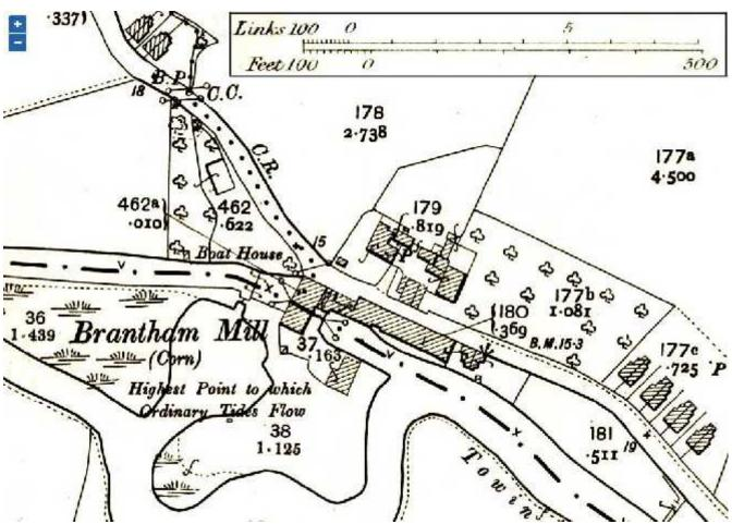
'The figures illustrate how 25-inch plans, despite being more out-of-date, were much more useful for planning rural sewerage than six-inch plans. Road levels, where shown, were closer together, and the delineation of individual properties provided an excellent basis for site inspections. At that time I was unaware of 'the battle of the scales' a century earlier, and I am impressed now to find that the
